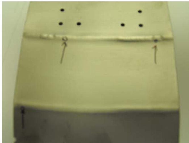
Figure 2. Face Side of Sample with Accumulated Pinholes within 1.70 Inches of the Length
