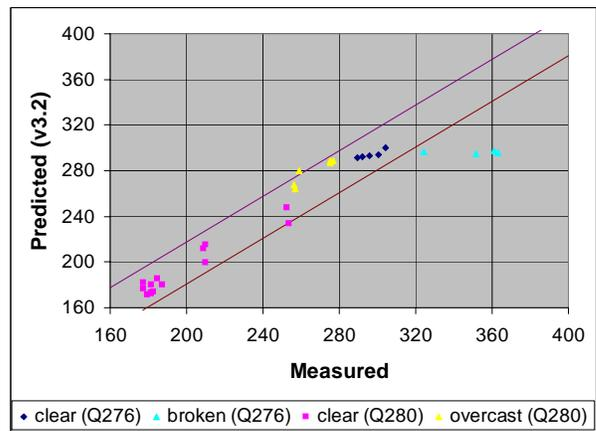
Figure 5: Down-welling thermal sky irradiance ( $\text{W/m}^2$ ).
