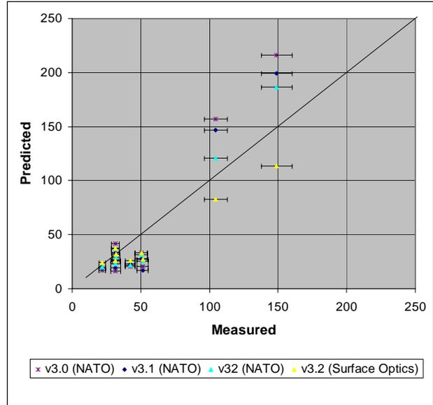
**Figure 9:** Predicted versus measured  $3\text{--}5\mu\text{m}$  ship signature (W/sr) for Q276 using different versions of NTCS and Quest paint properties.
