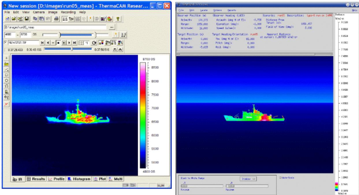
Figure 1: FLIR camera image of Quest taken during Q276 on left, with simulated output from ShipIR/NTCS (v3.2) on right.
