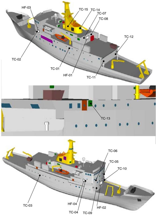
**Figure 3:** Thermocouple locations during Q280.
